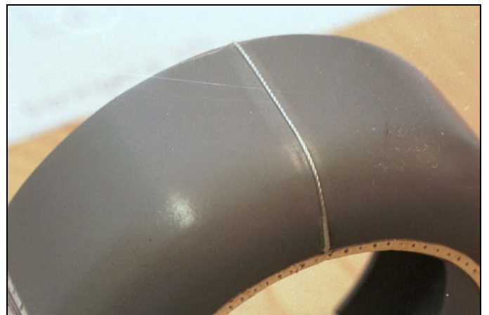
This was accomplished by first gluing a string to the cowl to simulate the ridge in the joint.
