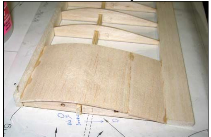
Lower Wing Sheeting
